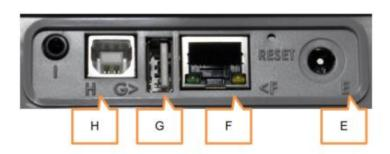
Those connectors are behind a trapdoor. It must remain close in industrial environment to preserve the IP65 protection. Use those connectors only in office environment.
